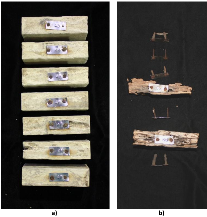
Figure 2: Condition of a) Accoya® Radiata and b) radiata pine sapwood test specimens after exposure to M. darwiniensis in a Hazard Class H3 field trial.
