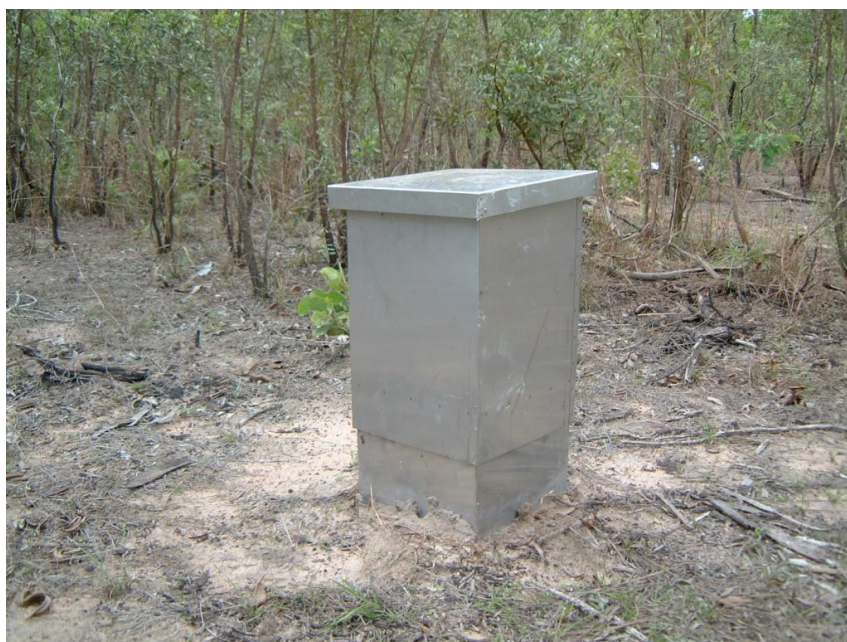
Figure 4: Exposure container containing test specimens and bait-wood, connected to active galleries of M. darwiniensis , prior to wrapping in sisalation to protect the contents against excessive heat and fire.
